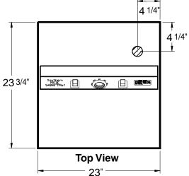
**Electrical Requirements:** 120 volts AC, 60 hertz, 1 phase, 20 amp wiring required. Construction: All 18 gauge Stainless Steel. Chipbox: Uses standard hardwood chips. **Dimensions:** 41 3/8" tall, 23" wide, 23 3/4" deep **Shell Dimensions:** 31 1/2" tall, 23" wide, 23 3/4"deep.
